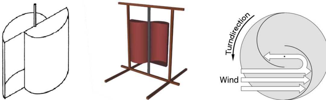
Fig. 2: Savonius rotor / wind power generator made out of oil barrels.
